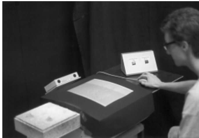
Figure 7.7. An overview of the experimental setup. The monitor with the virtual landscape is in front of the subject. The real landscape is on the left, the head tracker behind and the mouse and button box to the right of the monitor. A cardboard cover attached to the display served as a reduction screen.
