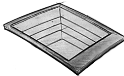
Figure 9.6b. With off-axis coupling the displayed planes stay parallel to the plane of the real display. In such cases where the real and displayed world are closely linked, off-axis coupling is more suitable than on-axis coupling.
