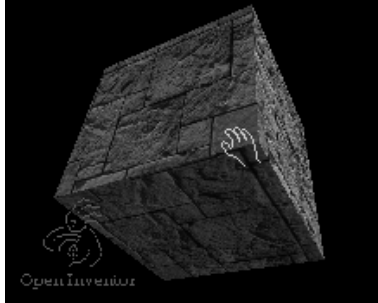
Figure 9.8a. A more intuitive way of selecting a view. Dragging the hand horizontally while it is in the middle of the window rotates the scene about the vertical axis.
