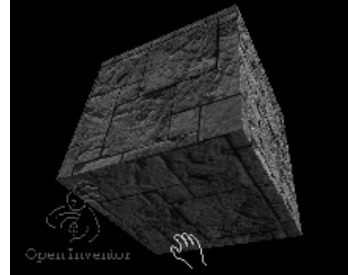
Figure 9.8b. If the hand is near the bottom of the window, dragging it horizontally results in a rotation of the scene around the axis out of the display.
