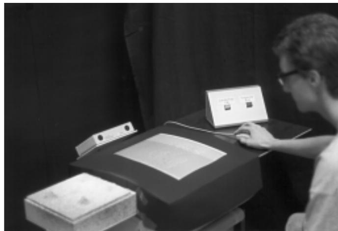
Figure 7.7. An overview of the experimental setup. The monitor with the virtual landscape is in front of the subject. The real landscape is on the left, the head tracker behind and the mouse and button box to the right of the monitor. A cardboard cover attached to the display served as a reduction screen.
