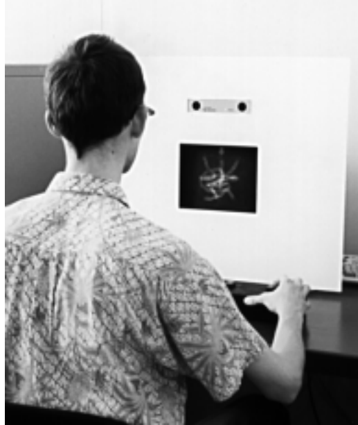
Figure 6.4. Overview of the experimental setup: a monitor with the eye position tracker on top of it and a reduction screen in front. The button box is below the monitor.
