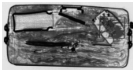
Figure 3.10 (see colour figure on left cover flap). Image from the CTX5000. Red indicates possible explosives, green parts of a detonator.
