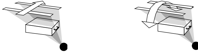
Figure 3.24. The movement of the x-ray source or sensor line can be a translation (left) or a rotation (right).
