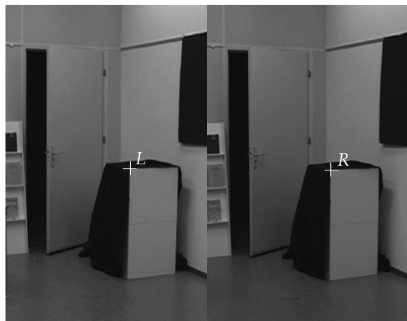
Figure 2.7. Image taken at left and right eye position. L and R are a matched position in these images, and they are expected to indicate a single position S in the spatial scene. This is a stereoscopic image, and can be viewed by looking at the left image with the left eye and at the right image with the right eye.
