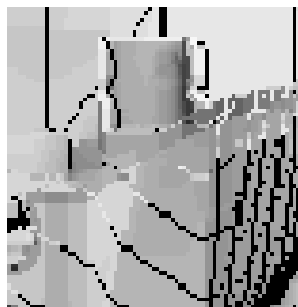
Figure 18b. Warped version of Figure 18a. Simple pixel copying will cause holes in the upscaled target image. (From Mark, McMillan and Bishop, 1997).
