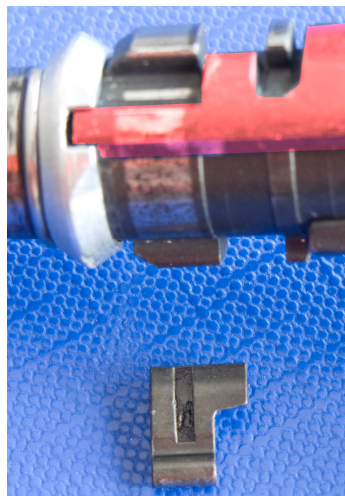
Figure 9. slots, control sleeve (in red) and pawl (at bottom). The pawl is shown in the same orientation as it would have if placed on the axle.
