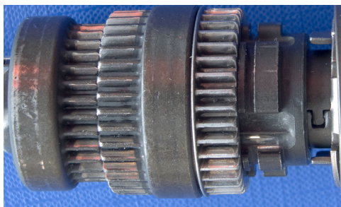
Figure 10. The three sun gears S4 , S3 and S2 (left to right) controlled by the control sleeve. S4 is captive inside planet cage 2.
