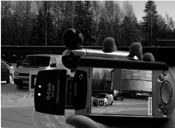
Figure 2. Fully equipped iPAQ in the outdoors demo (composite image). The camera is rotated physically to match the display used in landscape mode.
