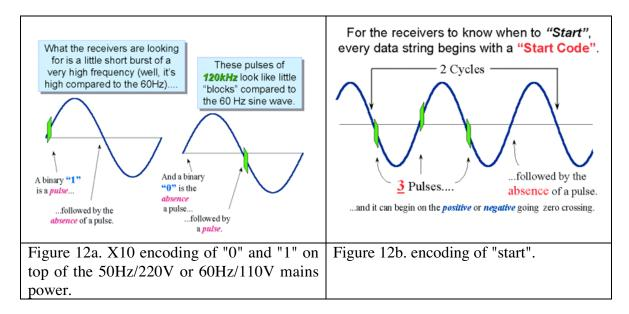
Not only the remote controls can inject signals onto the mains power, but also for instance video cameras, motion sensors, computers etc. A computer can then be used to control the whole system. X10 can also be controlled via radio or infrared, a special converter box (usually incorporated in a switch or dimmer module) is needed then.
