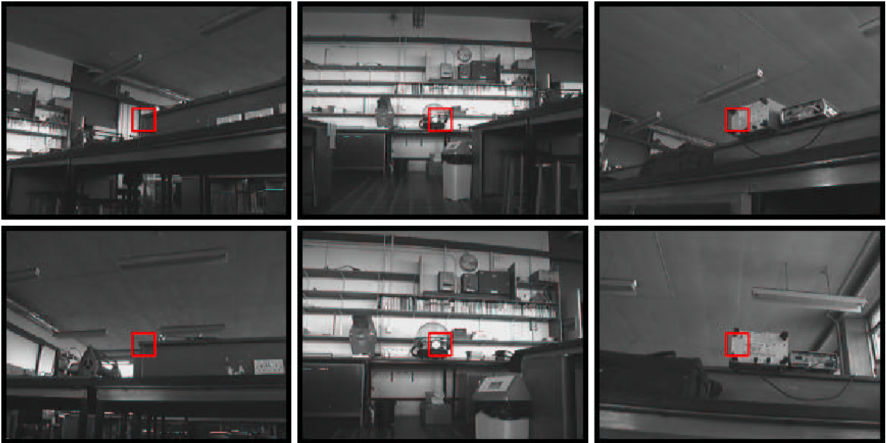
Figure 2. Automatically recognised and tracked templates (from [Davison99]). Red squares indicate template content and its real-world position.
