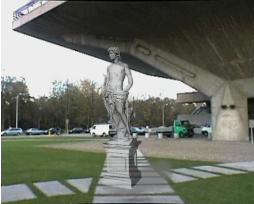
Figure 8. Preliminary nearby look at the statue. The statue is slightly transparent, due to the optical mixing of our AR system.
