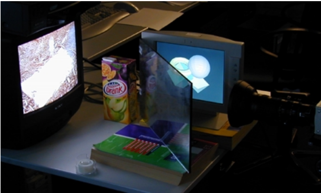
Figure 2. Prototype setup. On the left the PAL monitor. In the middle the half-transparent mirror, with the IBM VGA display behind it. At the right the Sony video camera. (The juice pack is just a safety measure in case the mirror might drop). Recording apparatus not shown.
