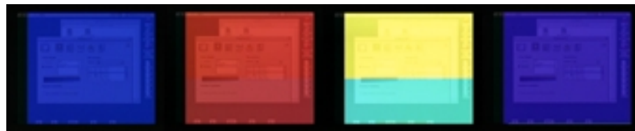
Figure 8. Snapshots from Roland V-5. Some frames are dropped entirely, here a green frame is dropped after the yellow frame.
