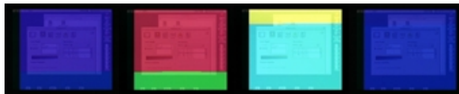
Figure 9. Sometimes frameparts are shown in reverse order. Here we see a fragment of a green frame displayed before a yellow is displayed.
