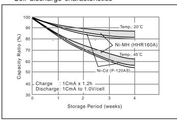
Self-discharge is affected by the temperature at which the batteries are left standing and the length of time during which they are left standing. It increases in proportion as the temperature or the shelf-standing time increases. Panasonic's nickel-metal hydride batteries have excellent self-discharge characteristics that are comparable to those of Ni-Cd batteries.
