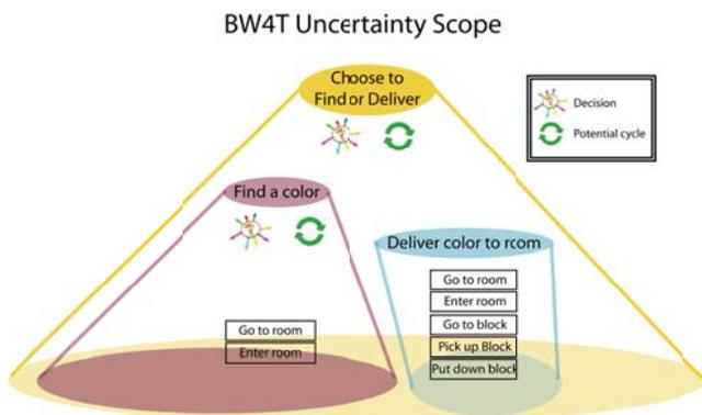
**Figure 4 Relative sizes of Uncertainty Scope for different aspects of BW4T algorithm. The delivery task has more activity, but less uncertainty than the find task, while the choice to find or deliver is broader in scope than both.**
