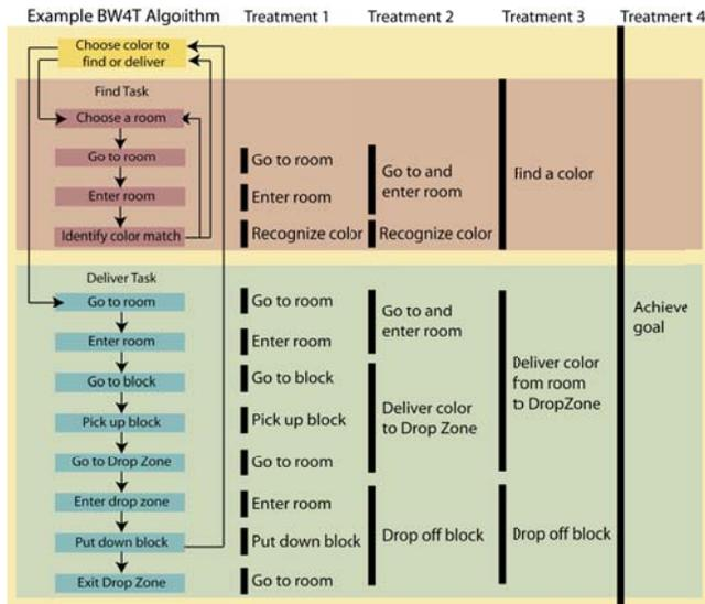
**Figure 3 Defining Autonomy Treatments for BW4T. The overall task (yellow box) can be thought of as being composed of several “find” tasks (red box) and several “deliver” tasks (blue box). These tasks are in turn composed of decision and action primitives.**
