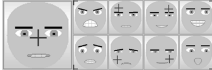
Figure 7: AffectButton and its different appearances while moving the cursor (the cross)
