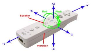
Figure 6 - Input sensors and output actuators of the Nintendo Wii Remote
