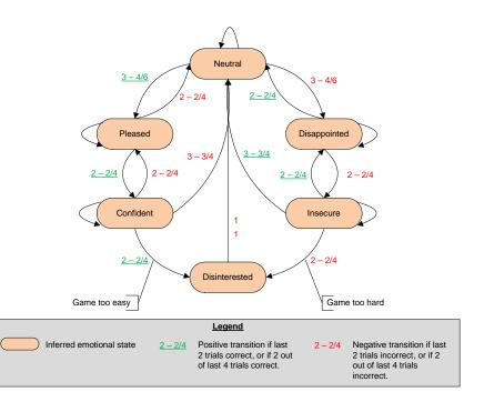
Figure 9 - Emotion knowledge base and the transitions triggered by semantic primitives for the input controller
