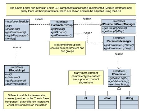
Figure 31 - High level overview of the Engine Core component
